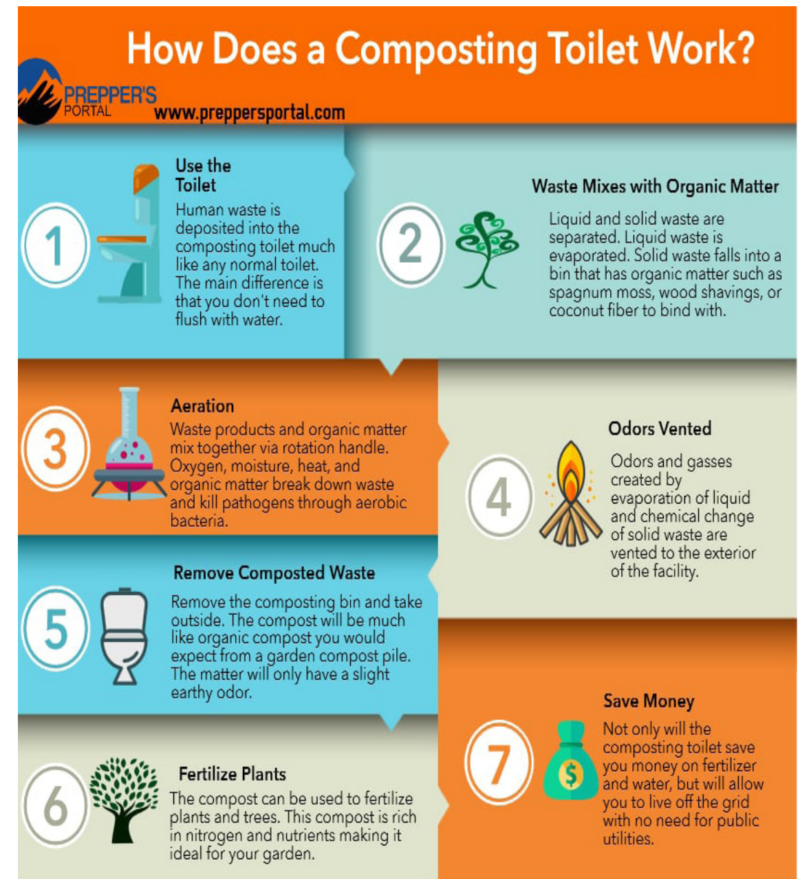
Figure 3. Basics on how a Dry (Composting) Toilet Works
