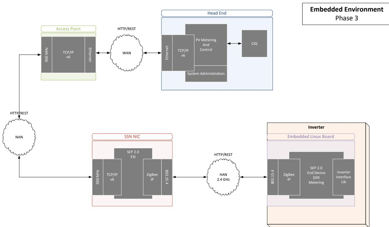
Figure 2. Embedded Environment - Inverter Deployment to the Embedded Environment [SSN SoW Task 1.3]
