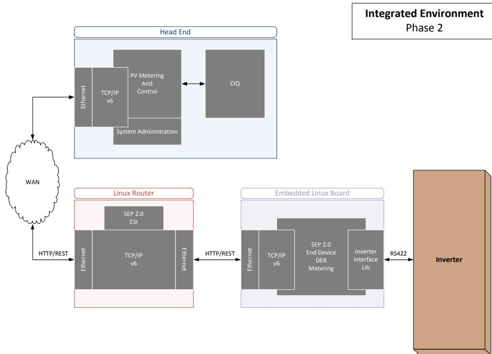
Figure 1. Integrated Environment - Inverter Deployment to the Integrated Environment [SSN SoW Task 1.2]
