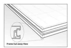
Zep System II is installed with Zep Compatible PV modules whose frames have been manufactured with the **Zep Groove**.
